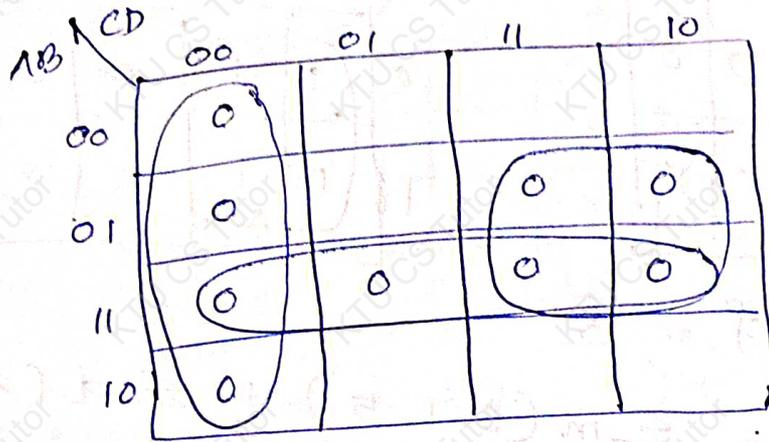
$$f = (C + D)(\bar{A} + \bar{B})(\bar{B} + \bar{C})$$
